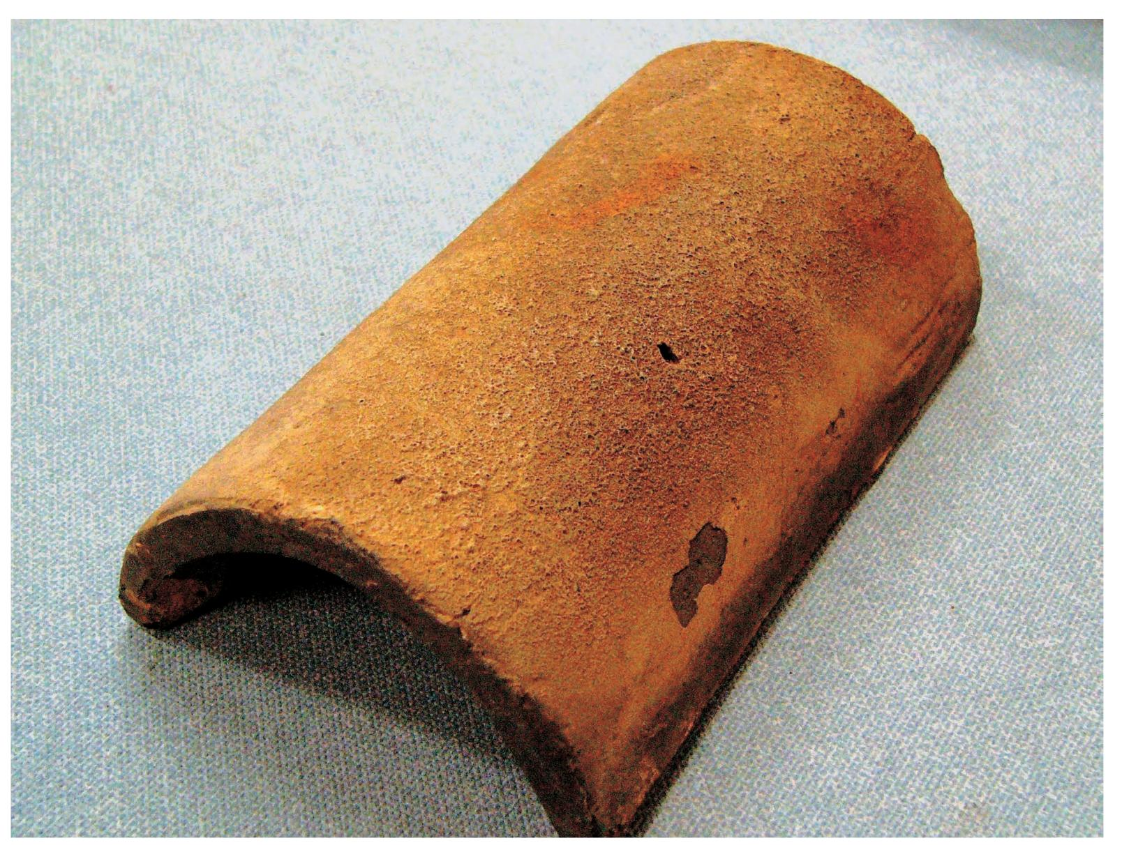
This tile was exposed to the atomic bomb causing the surface to boil and bubble. This phenomenon was confirmed in an experiment where tiles were exposed to heat measuring 1800 degrees Celsius for 4 seconds.
